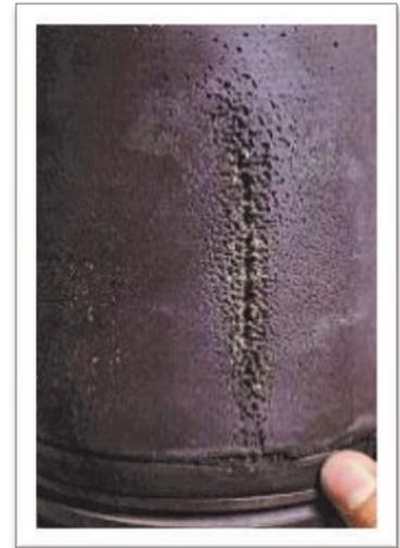
The bottom line is that changing your antifreeze on the manufacturer's time basis is important regardless of the hours of use in that period due to the fact that the inhibitors are being used up in their battle to prevent corrosion and cavitation.
