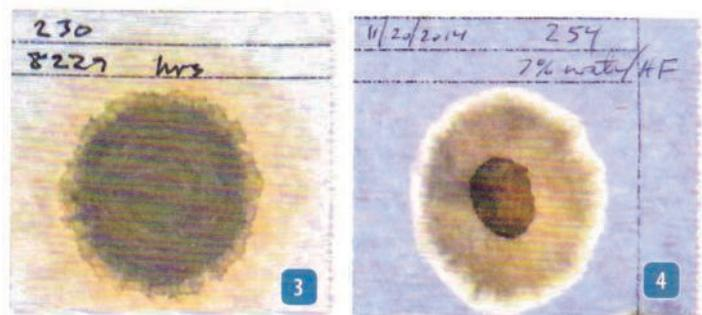
In a similar test, this second pair of pictures the first oil spot (#2), is from a healthy gasoline engine, and again the fine carbon combustion products spread quite widely with the engine oil as their carrier. The second picture (#3), is from an engine with a blown head gasket and the 10% antifreeze in oil mixture again clogs the paper pores and while the fuel still travels about the same, the combustion products don't.
